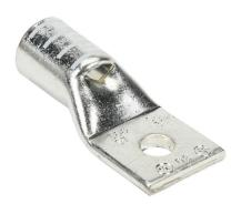
Penn-Union BLU series compression lug, standard barrel, tinplated copper, 35 kV, 3/8in mounting bolt, 1 hole, 300 MCM, white markings.
