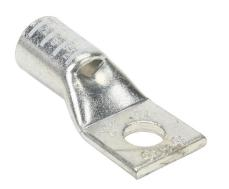
Penn-Union BLU series compression lug, standard barrel, tinplated copper, 35 kV, 1/2in mounting bolt, 1 hole, 300 MCM, white markings.
