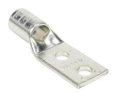
Penn-Union BLU series compression lug, standard barrel, tinplated copper, 35 kV, 3/8in mounting bolt, 2 hole, 1in hole spacing, 300 MCM, white markings.
