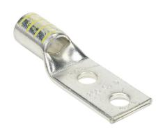
Penn-Union BLU series compression lug, standard barrel, tinplated copper, 35 kV, 3/8in mounting bolt, 2 hole, 1in hole spacing, 250 MCM, yellow markings.
