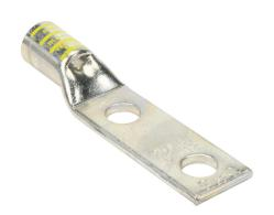
Penn-Union BLU series compression lug, standard barrel, tinplated copper, 35 kV, 1/2in mounting bolt, 2 hole, 1.75in hole spacing, 250 MCM, yellow markings.
