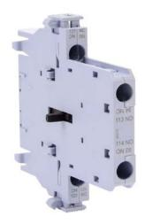
WEG Electric field installable auxiliary contact, side mount, (1) N.O./(1) N.C. contact(s), 1.5A @ 120 VAC/0.22A @ 120 VDC, screw terminal. For use with CWBx9 to CWBx125 series contactors.
