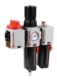
Norgren Excelon Plus 84 pneumatic combination unit, filter-regulator-lubricator, 3/4in female NPT inlet(s), 3/4in female NPT outlet(s), 4-145 psi range, die-cast aluminum bowl, automatic drain, manual shutoff valve.
