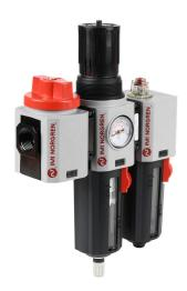
Norgren Excelon Plus 84 pneumatic combination unit, filter-regulator-lubricator, 3/4in female NPT inlet(s), 3/4in female NPT outlet(s), 4-145 psi range, polycarbonate bowl, automatic drain, manual shutoff valve.
