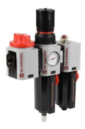
Norgren Excelon Plus 84 pneumatic combination unit, filter-regulator-lubricator, 1/2in female NPT inlet(s), 1/2in female NPT outlet(s), 4-145 psi range, die-cast aluminum bowl, automatic drain, manual shutoff valve.
