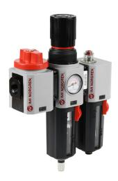
Norgren Excelon Plus 84 pneumatic combination unit, filter-regulator-lubricator, 1/2in female NPT inlet(s), 1/2in female NPT outlet(s), 4-145 psi range, polycarbonate bowl, automatic drain, manual shutoff valve.
