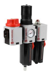
Norgren Excelon Plus 84 pneumatic combination unit, filterregulator-lubricator, 3/8in female NPT inlet(s), 3/8in female NPT outlet(s), 4-145 psi range, die-cast aluminum bowl, automatic drain, manual shutoff valve.
