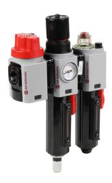
Norgren Excelon Plus 82 pneumatic combination unit, filter-regulator-lubricator, 3/8in female NPT inlet(s), 3/8in female NPT outlet(s), 4-145 psi range, die-cast zinc bowl, automatic drain, manual shutoff valve.
