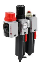
Norgren Excelon Plus 82 pneumatic combination unit, filter-regulator-lubricator, 3/8in female NPT inlet(s), 3/8in female NPT outlet(s), 4-145 psi range, polycarbonate bowl, manual drain, manual shutoff valve.
