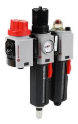
Norgren Excelon Plus 82 pneumatic combination unit, filterregulator-lubricator, 3/8in female NPT inlet(s), 3/8in female NPT outlet(s), 4-145 psi range, polycarbonate bowl, automatic drain, manual shutoff valve.
