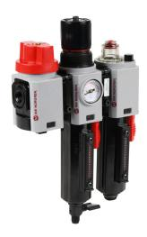
Norgren Excelon Plus 82 pneumatic combination unit, filter-regulator-lubricator, 1/4in female NPT inlet(s), 1/4in female NPT outlet(s), 4-145 psi range, die-cast zinc bowl, manual drain, manual shutoff valve.
