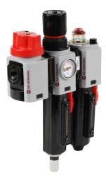
Norgren Excelon Plus 82 pneumatic combination unit, filterregulator-lubricator, 1/4in female NPT inlet(s), 1/4in female NPT outlet(s), 4-145 psi range, die-cast zinc bowl, automatic drain, manual shutoff valve.
