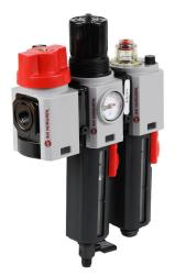
Norgren Excelon Plus 82 pneumatic combination unit, filterregulator-lubricator, 1/4in female NPT inlet(s), 1/4in female NPT outlet(s), 4-145 psi range, polycarbonate bowl, manual drain, manual shutoff valve.
