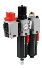
Norgren Excelon Plus 82 pneumatic combination unit, filter-regulator-lubricator, 1/4in female NPT inlet(s), 1/4in female NPT outlet(s), 4-145 psi range, polycarbonate bowl, automatic drain, manual shutoff valve.
