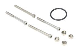
CITO long outlet mounting kit, for use with CITO StackFlow valves, includes (4) 1/4-20x2-1/4 SHCS, (4) 1/4-20 nuts and (1) O-ring.
