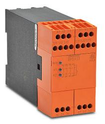
Dold safety relay, two-hand control, 2-channel, 110 VAC, (3) N.O. safety output(s), (1) N.C. monitoring output(s), fixed screw terminals.
