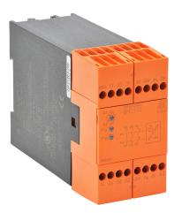
Dold safety relay, speed monitoring, (2) PNP sensor inputs, 2-channel, 24 VAC/VDC, (2) N.O. and (1) N.C. safety output(s), fixed screw terminals.
