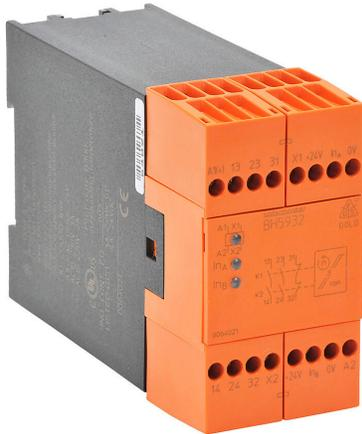
Dold safety relay, speed monitoring, (2) PNP sensor inputs, 2-channel, 24 VAC/VDC, (2) N.O. and (1) N.C. safety output(s), fixed screw terminals.
