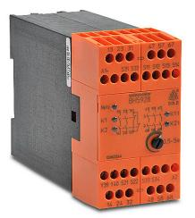
Dold safety relay, emergency stop and safety gates, release delay, 0.5 to 5 seconds, 2-channel, 24 VAC/VDC, (3) N.O. time delay and (2) N.O. safety output(s), (1) N.C. monitoring output(s), fixed screw terminals.
