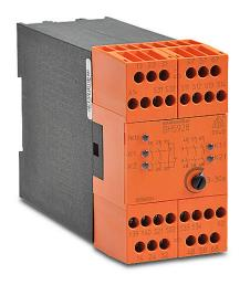
Dold safety relay, emergency stop and safety gates, release delay, 3 to 30 seconds, 2-channel, 24 VAC/VDC, (3) N.O. time delay and (2) N.O. safety output(s), (1) N.C. monitoring output(s), fixed screw terminals.
