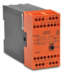
Dold safety relay, emergency stop and safety gates, release delay, 0.1 to 1 second, 2-channel, 24 VAC/VDC, (3) N.O. time delay and (2) N.O. safety output(s), (1) N.C. monitoring output(s), fixed screw terminals.
