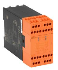
Dold safety relay, light curtain controller, 2-channel, 24 VDC, (2) N.O. safety output(s), (1) N.C. monitoring output(s), fixed screw terminals.
