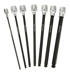
Bondhus ProHold impact socket bit set, external hex, 7 pieces, protanium high torque steel, 6in bit length, 1/4in drive, imperial, ball-end tip.
