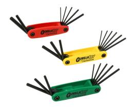
Bondhus GorillaGrip fold-out hex and torx key set, external hex and Torx, 24 pieces, 4.5in (114mm) overall length, protanium high torque steel, imperial and metric.
