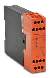
Dold safety relay, two-hand control, 2-channel, 24 VDC, (2) N.O. safety output(s), (1) N.C. monitoring output(s), fixed screw terminals.
