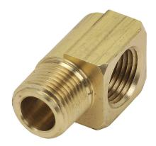
NITRA pneumatic threaded fitting, street elbow, brass body, 3/8in female NPT to 3/8 male NPT. Package of 2.
