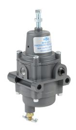
NITRA precision pneumatic filter-regulator, 1/4in female NPT inlet(s), 1/4in female NPT outlet(s), 0-30 psi adjustable range, manual drain, die-cast aluminum bowl, sight gauge.
