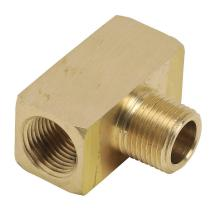
NITRA pneumatic threaded fitting, tee, brass body, (1) 3/8in male NPT to (2) 3/8in female NPT. Package of 2.
