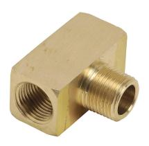
NITRA pneumatic threaded fitting, tee, brass body, brass threads, (1) 1/8in male NPT to (2) 1/8in female NPT. Package of 2.
