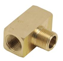
NITRA pneumatic threaded fitting, tee, brass body, brass threads, (1) 1/4in male NPT to (2) 1/4in female NPT. Package of 2.
