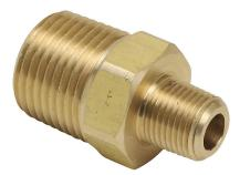
NITRA pneumatic threaded fitting, straight, brass body, brass threads, (1) 3/8in male NPT to (1) 1/8in male NPT. Package of 5.
