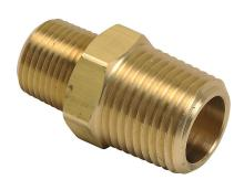
NITRA pneumatic threaded fitting, straight, brass body, 1/2in male NPT to 3/8in male NPT. Package of 2.
