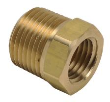
NITRA pneumatic threaded fitting, hex bushing, brass body, brass threads, (1) 3/8in male NPT to (1) 1/4in female NPT. Package of 5.
