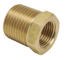
NITRA pneumatic threaded fitting, hex bushing, brass body, brass threads, (1) 1/2in male NPT to (1) 3/8in female NPT. Package of 2.
