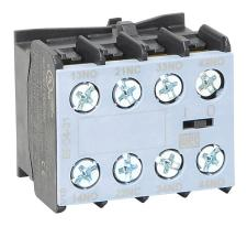
WEG Electric auxiliary contact, front mount, (3) N.O./(1) N.C. contact(s), 6A @ 120 VAC/0.55A @ 120 VDC. For use with any 4-pole CWC07 through CWC016 series miniature contactor with standard consumption AC or DC coils.
