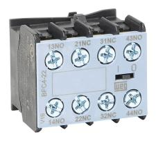
WEG Electric auxiliary contact, front mount, (2) N.O./(2) N.C. contact(s), 6A @ 120 VAC/0.55A @ 120 VDC. For use with any 4-pole CWC07 through CWC016 series miniature contactor with standard consumption AC or DC coils.
