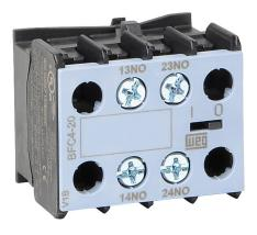
WEG Electric auxiliary contact, front mount, (2) N.O. contact(s), 6A @ 120 VAC/0.55A @ 120 VDC. For use with any 4-pole CWC07 through CWC016 series miniature contactor.
