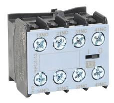
WEG Electric auxiliary contact, front mount, (1) N.O./(3) N.C. contact(s), 6A @ 120 VAC/0.55A @ 120 VDC. For use with any 4-pole CWC07 through CWC016 series miniature contactor with standard consumption AC or DC coils.
