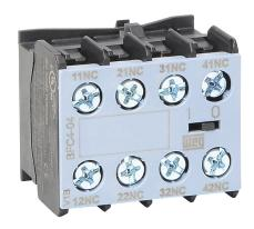
WEG Electric auxiliary contact, front mount, (4) N.C. contact(s), 6A @ 120 VAC/0.55A @ 120 VDC. For use with any 4-pole CWC07 through CWC016 series miniature contactor with standard consumption AC or DC coils.
