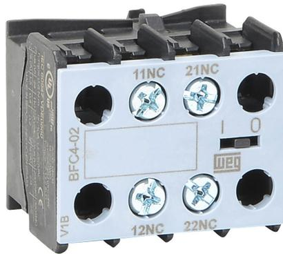
WEG Electric auxiliary contact, front mount, (2) N.C. contact(s), 6A @ 120 VAC/0.55A @ 120 VDC. For use with any 4-pole CWC07 through CWC016 series miniature contactor.
