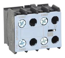
WEG Electric auxiliary contact, front mount, (2) N.O. contact(s), 6A @ 120 VAC/0.55A @ 120 VDC. For use with any 3-pole CWC025 series miniature contactor.
