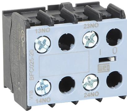
WEG Electric auxiliary contact, front mount, (2) N.O. contact(s), 6A @ 120 VAC/0.55A @ 120 VDC. For use with any 3-pole CWC025 series miniature contactor.
