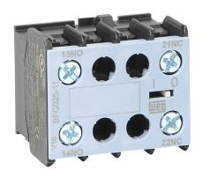
WEG Electric auxiliary contact, front mount, (1) N.O./(1) N.C. contact(s), 6A @ 120 VAC/0.55A @ 120 VDC. For use with any 3-pole CWC025 series miniature contactor.
