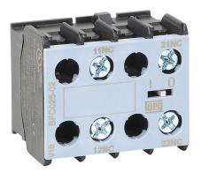
WEG Electric auxiliary contact, front mount, (2) N.C. contact(s), 6A @ 120 VAC/0.55A @ 120 VDC. For use with any 3-pole CWC025 series miniature contactor.
