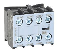
WEG Electric auxiliary contact, front mount, (4) N.O. contact(s), 6A @ 120 VAC/0.55A @ 120 VDC. For use with any 3-pole CWC07 through CWC016 series miniature contactor with standard consumption AC or DC coils.
