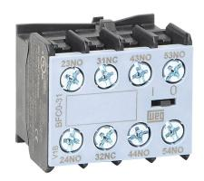
WEG Electric auxiliary contact, front mount, (3) N.O./(1) N.C. contact(s), 6A @ 120 VAC/0.55A @ 120 VDC. For use with any 3-pole CWC07 through CWC016 series miniature contactor with standard consumption AC or DC coils.
