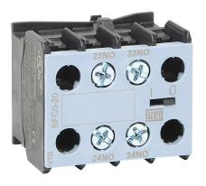
WEG Electric auxiliary contact, front mount, (2) N.O. contact(s), 6A @ 120 VAC/0.55A @ 120 VDC. For use with any 3-pole CWC07 through CWC016 series miniature contactor.
