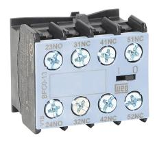
WEG Electric auxiliary contact, front mount, (1) N.O./(3) N.C. contact(s), 6A @ 120 VAC/0.55A @ 120 VDC. For use with any 3-pole CWC07 through CWC016 series miniature contactor with standard consumption AC or DC coils.
